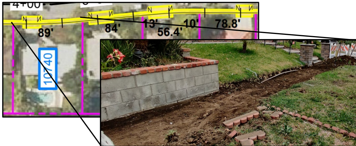
Figure 9. Early Design Plans Often Call for Sidewalk Removal Along the Entire Path of Travel
